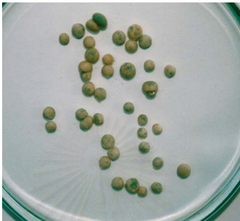
Figure 4.11 Chitosan Coated Fertilizer in Deionized Water at Zero Minute.
