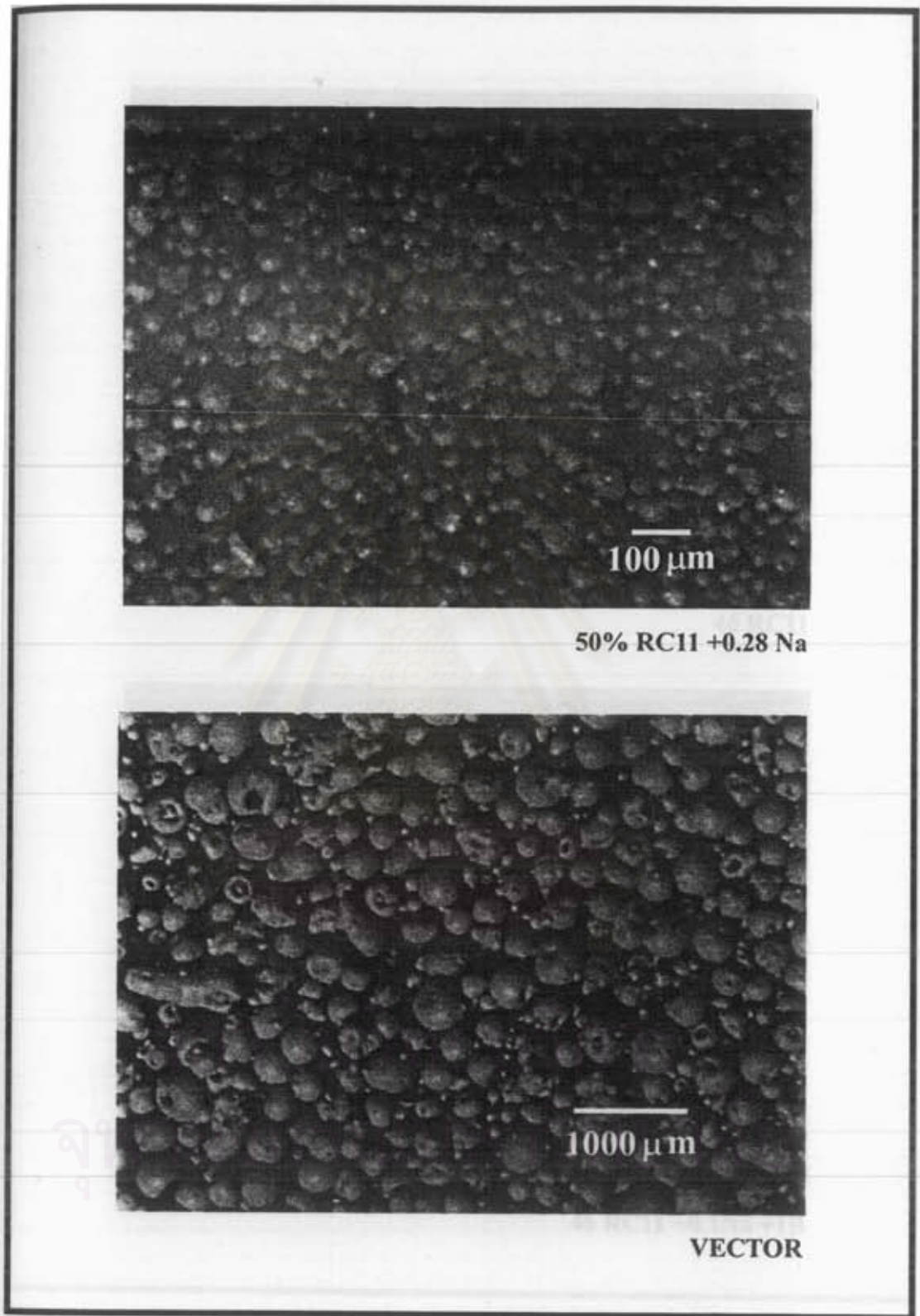
Fig. 5.33 Granule figures of 50%RC11+ 0.28 wt% \text{Na}_2\text{SiO}_3 (Varied condition) and Hypure Vector ® by stereomicroscope
