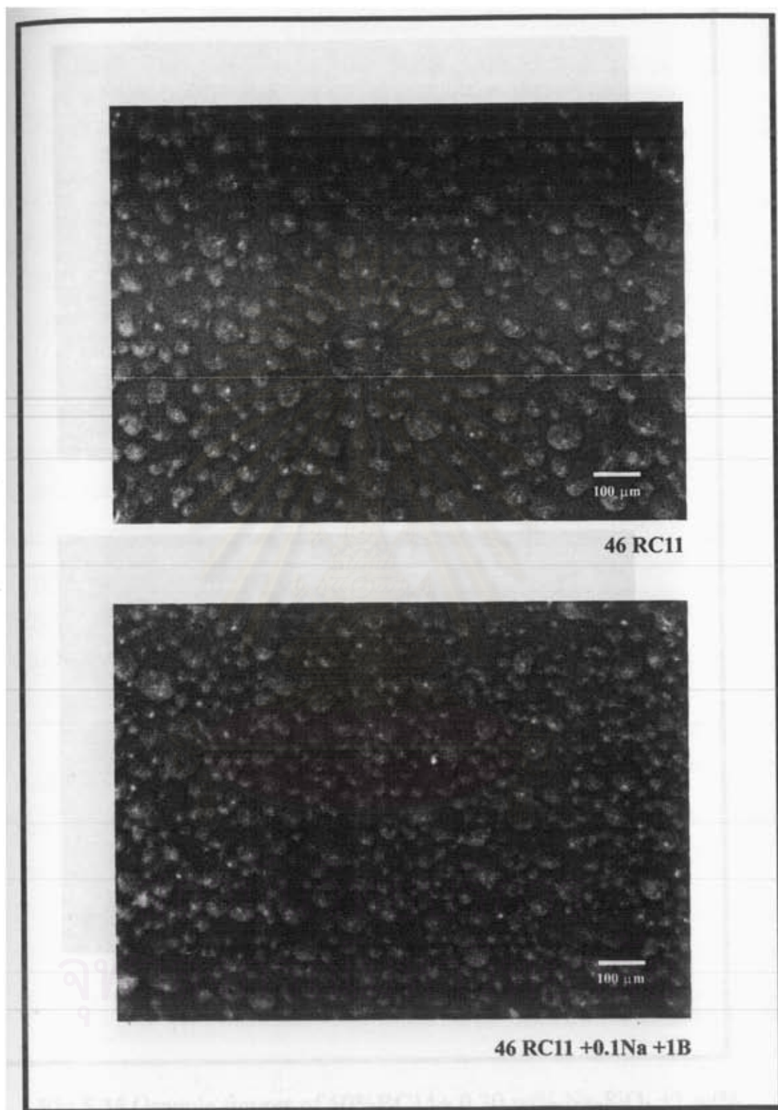
Fig. 5.34 Granule figures of 46%RC11 and 46%RC11+1 wt% binder + 0.10 wt% \text{Na}_2\text{SiO}_3 (Varied condition) by stereomicroscope
