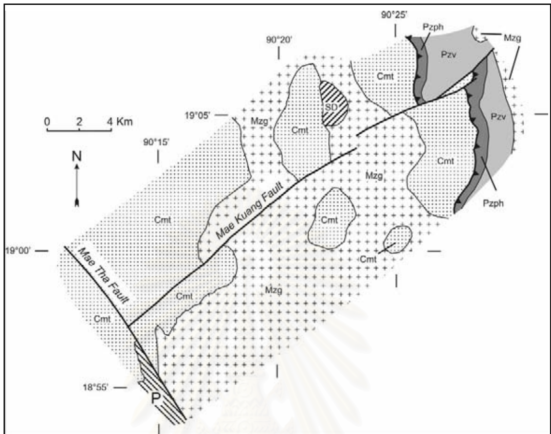
Figure 1.18 Geologic map along the trace of the Mae Kuang fault. P, undifferentiated Permian rocks; Cmt, Mae Tha Formation; SD, Silurian and Devonian Rocks; Pzph, Paleozoic phyllite; Pzv, Paleozoic metabasalt; Mzg, granitic rocks of the Fang-Mae Suai batholith. (After Rhodes et al., 2002).
