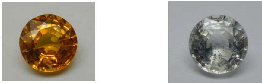
Figure 4.3 A heat-treated sapphire (PC3) shows strong yellow before experiment (left) and becomes colourless (right) after reheating at 1,650 °C in N 2 atmosphere for 5 hours
