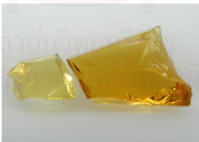
Figure 6.1 Comparison of the colour of sample YCH1 before treatment (the smaller reference sample on the left) with that (the larger sample on the right) after heat treatment at high temperature in an oxidizing condition
