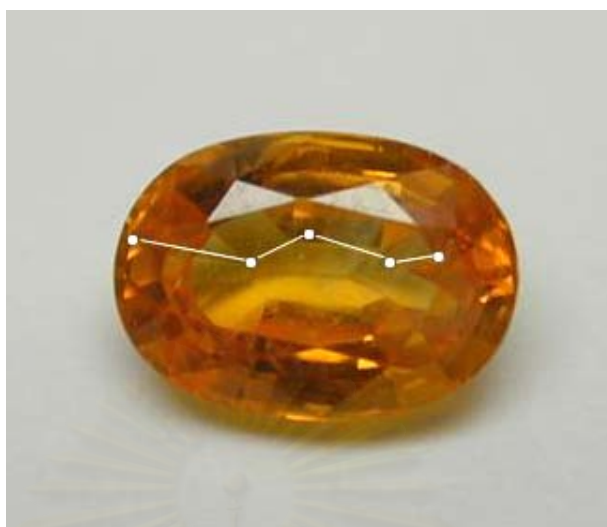
Figure 4.18 Close-up view of the sample PC2 showing the locations of the five point analyses from left to right by LA-ICP-MS.
