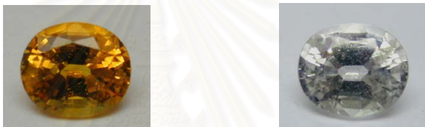
Figure 4.4 A heat-treated sapphire (PC4) shows strong yellow before experiment (left) and becomes colourless (right) after reheating at 1,650 °C in N 2 atmosphere for 5 hours
