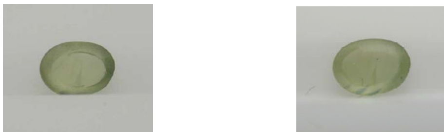
Figure 5.7 A light yellowish green sapphire with blue zones (CH7) before treatment (left) does not show any change in colour after heating at 1,650 °C in O 2 atmosphere for 24 hours (right).
