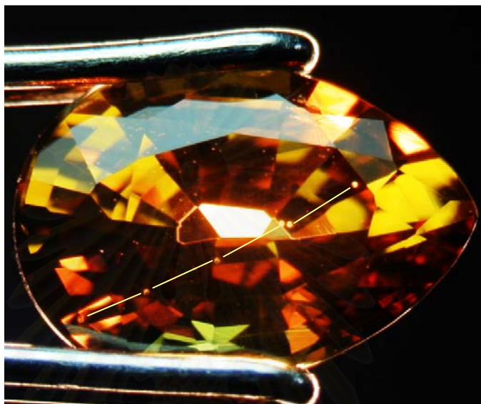
Figure 6.9 Close-up view of the sample YCH2 showing the approximate locations of the five point analyses from left to right by LA-ICP-MS.
