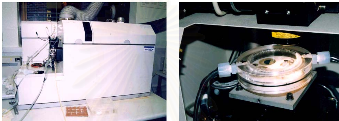
Figure 2.5 Laser Ablation Inductively-Coupled-Plasma Mass Spectrometry (LA-ICP-MS) at the Macquarie University in Sydney, Australia
