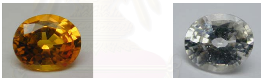
Figure 4.1 A heat-treated sapphire (PC1) shows strong yellow before experiment (left) and becomes colourless (right) after re-heating at 1,650 °C in N 2 atmosphere for 5 hours
