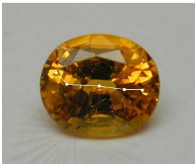
Figure 4.22 Close-up view of the sample PC4 showing the locations of the five point analyses from left to right by LA-ICP-MS.
