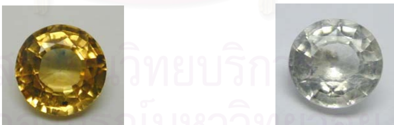
Figure 4.5 A heat-treated sapphire (PC5) shows medium yellow before experiment (left) and becomes colourless (right) after reheating at 1,650 °C in N 2 atmosphere for 5 hours
