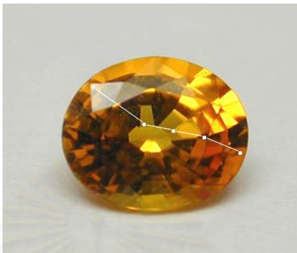
Figure 4.16 Close-up view of the sample PC1 showing the locations of the five point analyses from left to right by LA-ICP-MS.
