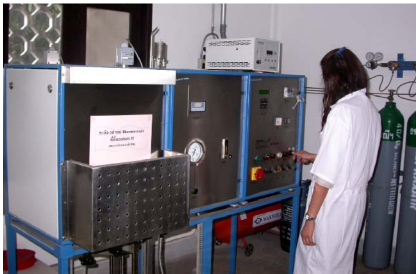
Figure 2.3 Linn electrical furnace model HT 1800 Plus VAC Bottom Loader based at the Department of Geology, Faculty of Science, Chulalongkorn University.
