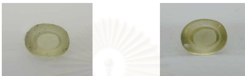
Figure 5.1 A very light yellow sapphire (CH1) before treatment (left) does not show any change in colour after heating at 1,650 °C in O 2 atmosphere for 24 hours (right).
