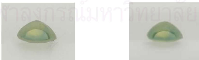
Figure 5.3 A light greenish yellow sapphire with blue zones (CH3) before treatment (left) does not show any change in colour after heating at 1,650 °C in O 2 atmosphere for 24 hours (right).
