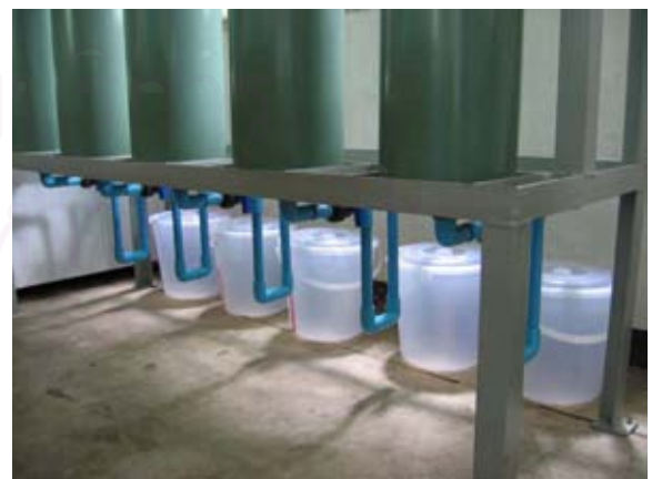
(c) Effluent pipe and Leachate container
