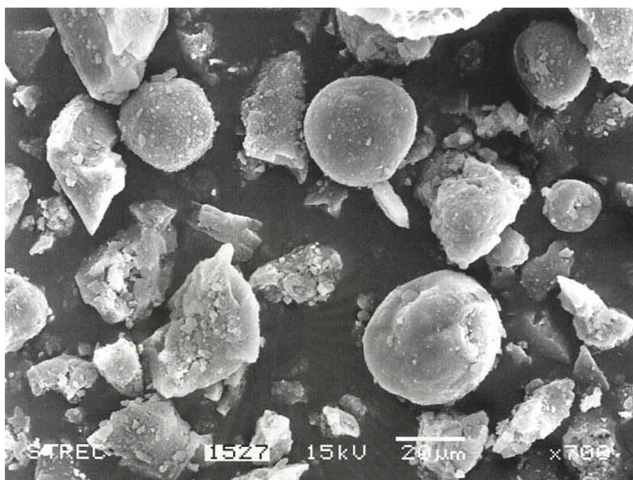
Figure 4.14 Scanning electron microscope image of silica/MAO/Et(Ind) 2 ZrCl 2
