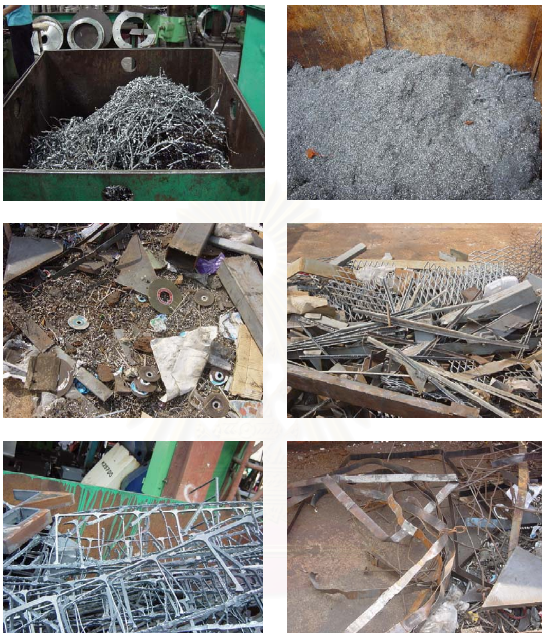
Figure 4.33 Shape of steel scrap in New Bang Poo Manufacturing Co., Ltd.
