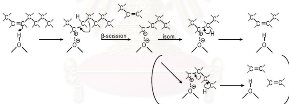
Figure 2.13 Monomolecular cracking mechanisms with ZSM-5.
