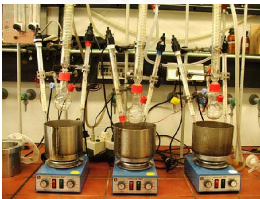
Figure 3.1 The experimental setup for round bottom flask reactor.
