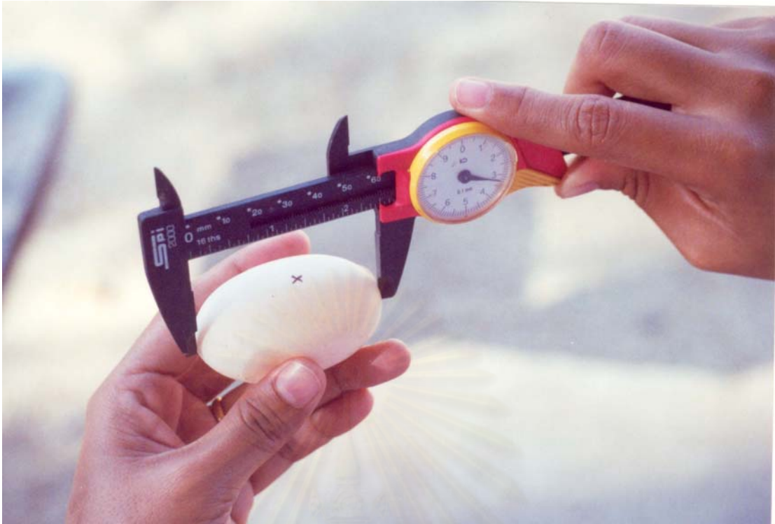
Figure 7: Measuring Batagur baska egg with a dial caliper at Bota Kanan Hatchery in Perak Malaysia.
