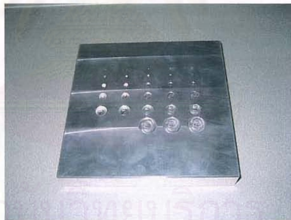
Figure 3.5 PortalVision ATP Phantom (Portal Vision TM , Varian medical system).
