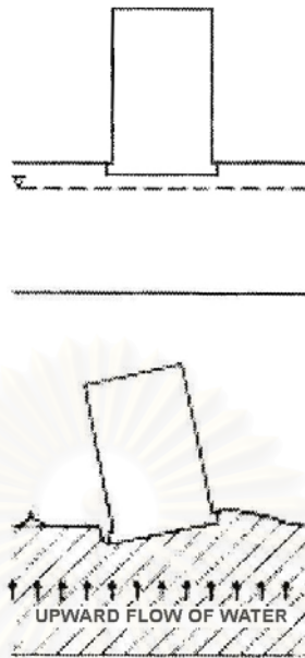
Fig. 2.25. Example of structure tilted due to loss of bearing strength. Liquefaction weakens the soil reducing foundation support which allows heavy structures to settle and tip.
