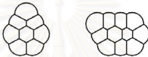
Figure 4.2.9: Some 5-bubbles with one or two hexagonal components.
