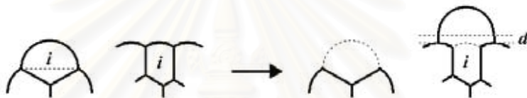
Figure 4.1.9: A bubble with a 3-sided component and a 5-sided component of R_i can be improved to a shorter enclosure.
