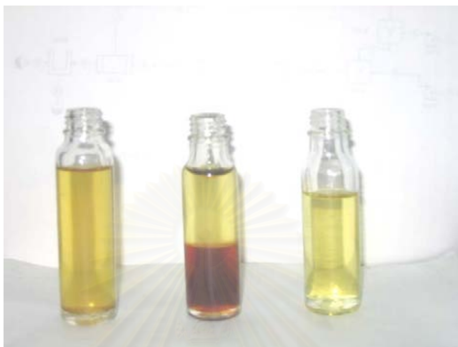
Figure 4.11 Picture of used palm oil (left), glycerol (middle), and methyl esters (right)
