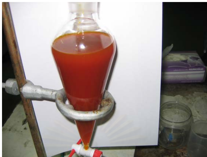
Figure 4.13 Picture of crude palm oil after reaction standing overnight to insure the separation of the methyl ester (biodiesel)
