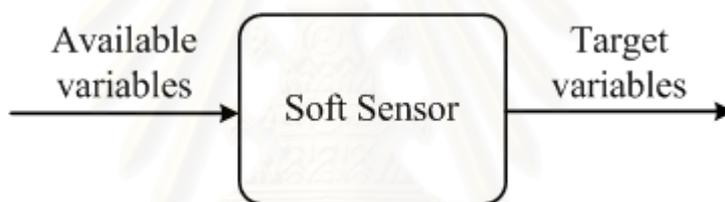
Figure 2.1: The structure of soft sensor.
