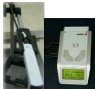
Figure 3.8. Solid state dosimeter UNFORS model Xi
