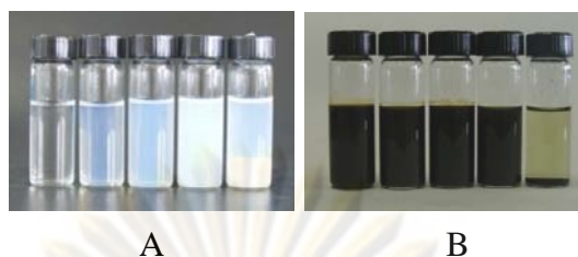
Figure 4.6 The photographic images of (A) Silver citrate complex that had [trisodium citrate]/[AgNO 3 ] from 4.0 \times 10^{-3} , 8.0 \times 10^{-3} , 1.6 \times 10^{-2} , and 3.2 \times 10^{-2} , respectively and (B) silver nanoparticles were synthesized from silver citrate complex with NaBH 4 .
