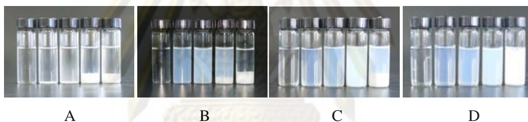
Figure 4.5 Silver citrate complex at various concentration (A) without starch, (B) 0.10 % (w/v), (C) 0.25 % (w/v), and (D) 0.50 % (w/v) starch. The molar ratio of trisodium citrate dihydrate to silver nitrate, [\text{trisodium citrate}]/[\text{AgNO}_3] was increased from 0, 4.0 \times 10^{-3} , 8.0 \times 10^{-3} , 1.6 \times 10^{-2} , and 3.2 \times 10^{-2} , respectively.
