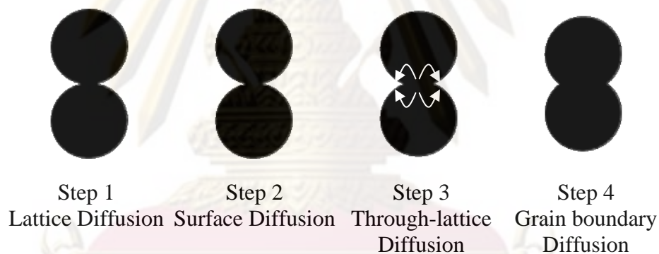
Figure 2.4 Schematic diagram of diffusion step between two particles, step 1 and 2 are lattice and surface diffusion mechanisms, respectively. These two steps do not produce any shrinkage. Step 3 and 4 are densification, center of particles approach to one another. These two steps are through-lattice diffusion and grain boundary diffusion.
