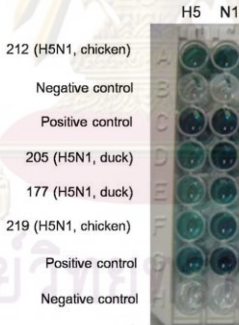
Figure 10: Identification of influenza A virus subtype H5N1 by PCR-ELISA. Positive M, H5, and N1 genes were identified as increasing of color intensity ( O.D_{.405} - O.D_{.492} > 0.3 ).
