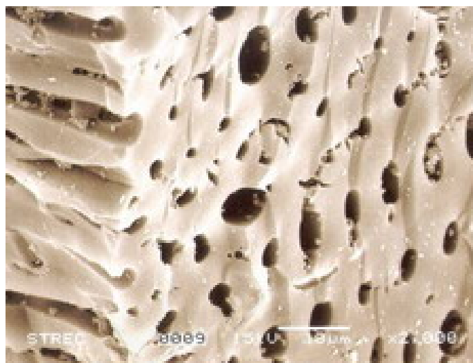
Figure 4.1 SEM photomicrograph of powdered activated carbon
