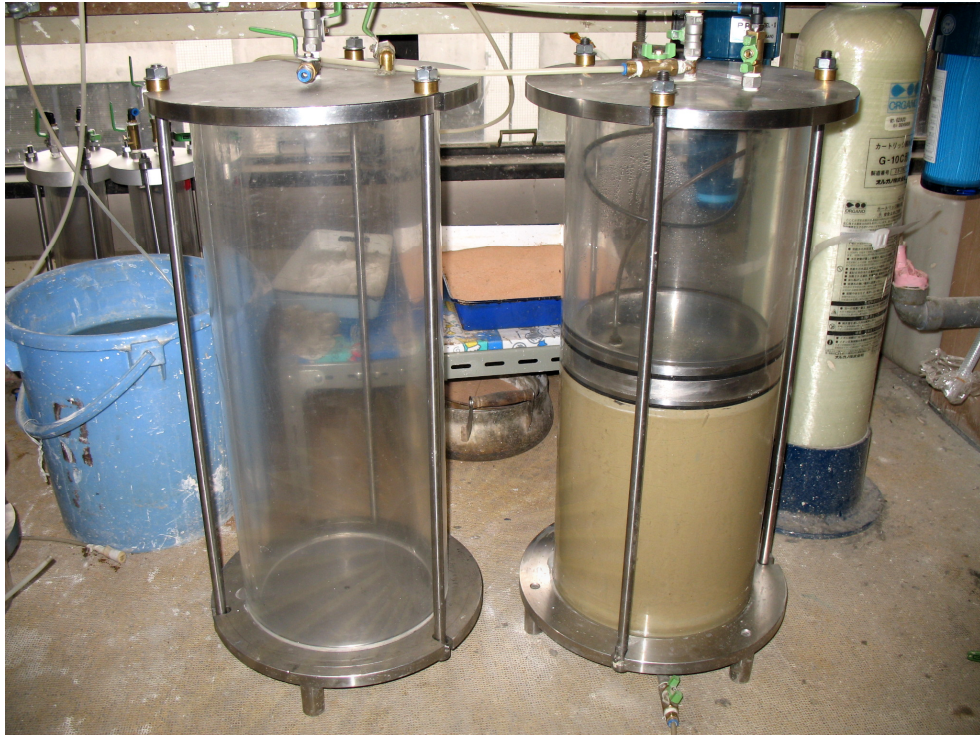
Figure 3.7 The slurry is preconsolidated under vertical pressure in preconsolidation cell.
