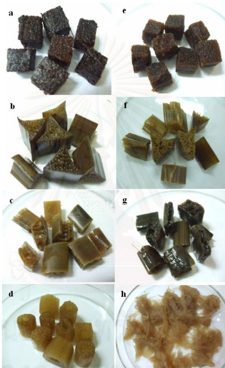
Figure 4.1 Structure of undelignified (a = coir, b = bulrush, c = banana stem, d = water hyacinth stem) and delignified (e = coir, f = bulrush, g = banana stem, h = water hyacinth stem) support material.
