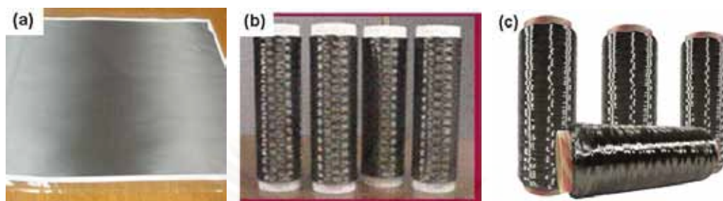
Figure 2.4 Various types of fibers; (a) boron fiber (b) silicon carbide (SiC) fiber and (c) carbon fiber (CF).
