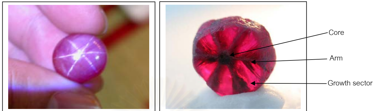
Figure 1.1 Characteristic of a star ruby (left) compared with a trapiche ruby (right) (right photo from www. crystal-treasure.com ).
