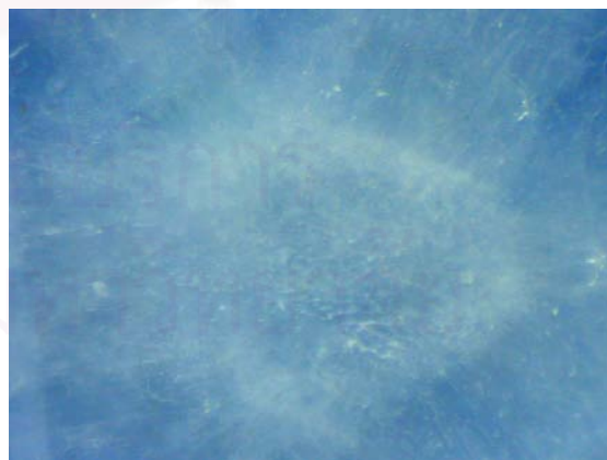
Figure 4.3.3 Internal features observed in Pailin2 (C2) showing well developed hexagonal core (70x) containing very tiny inclusions of thin-film fluid and minute particles
