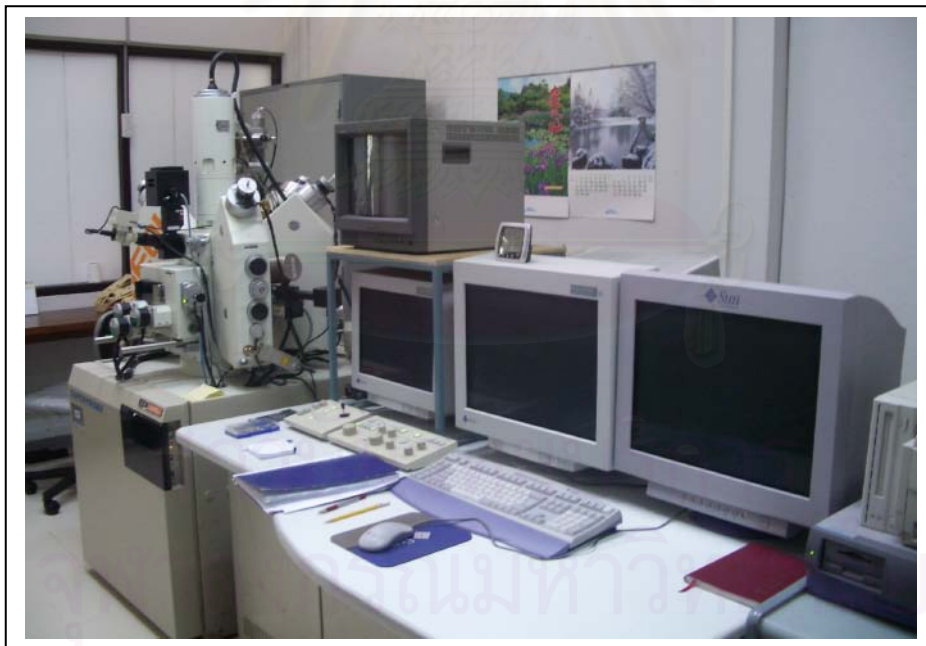
Figure 3.2 Electron Probe Micro-Analyzer (EPMA) based at the Department of Geology, Chulalongkorn University.
