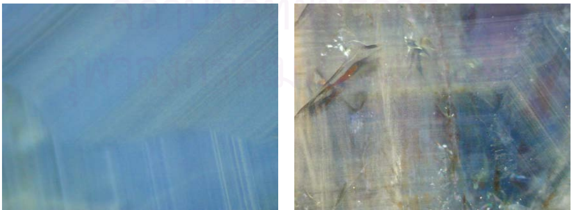
Figure 4.4.5 Internal features observed around growth sectors of trapiche sapphires from Vietnam showing clouds of fine minute particles along growth zones (70x) of Di Linh_O1 (left) and blue growth sector with mainly thin-film fluid inclusions and minute particles along growth zones (20x) in Di Linh_H.
