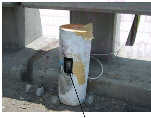
Photoelectric sensors (6.5cm x2cm)
