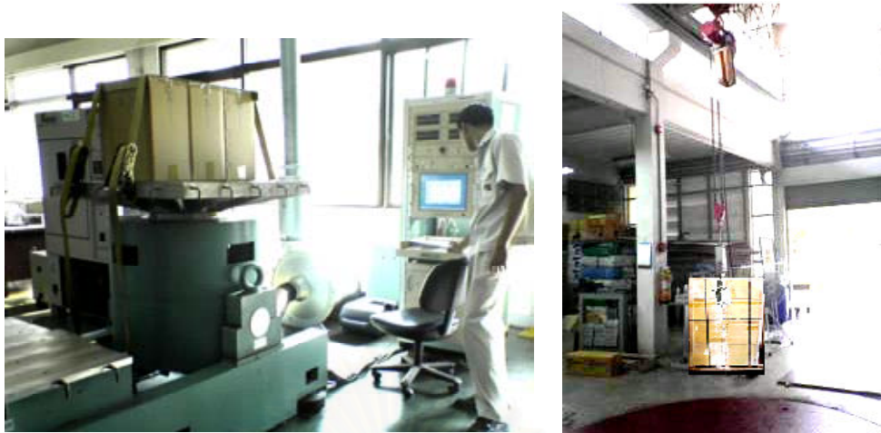
Figure 2.9 Vibration Tester at Thai Automotive Institute and Drop test at Thai Packaging Centre
