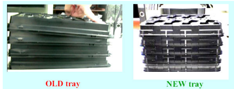
Figure 5.24 Stacking feature of HSA tray
