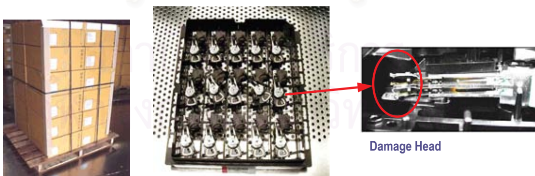
Figure 1.3 HSA Defect from Handling and Transportation
