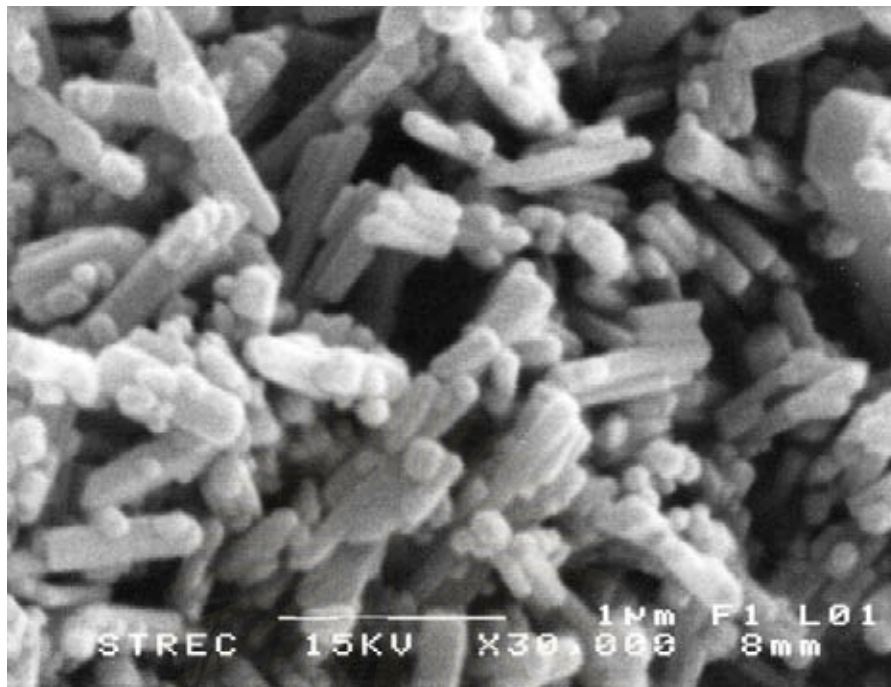
Figure 5.10 SEM images of ZnO nanoparticles as-synthesized in 1-octanol at 250 °C for 2 h by using zinc acetate 15 g.
