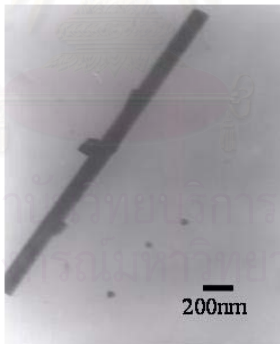
Figure 5.61 TEM image of ZnO nanoparticles as-synthesized in toluene at 300°C for 2 h by using zinc acetate 20 g.
