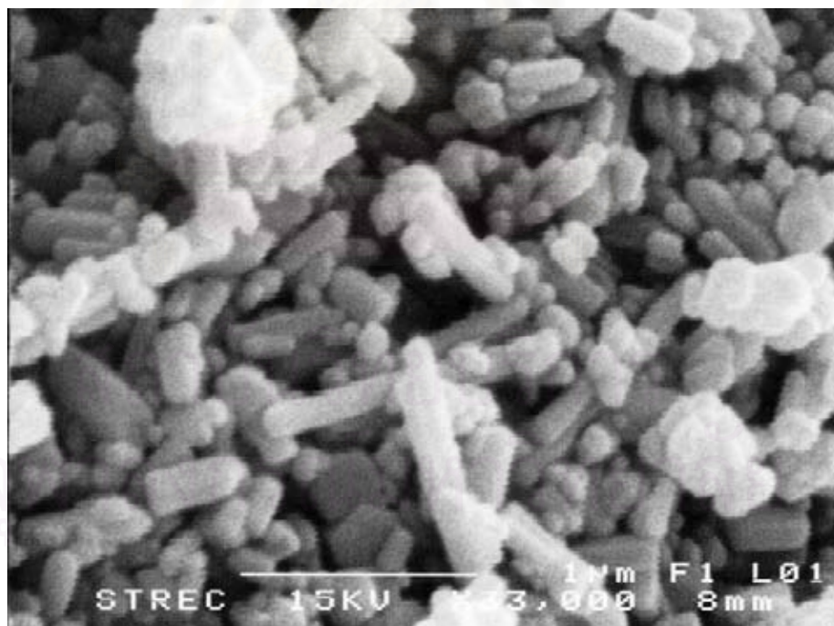
Figure 5.9 SEM images of ZnO nanoparticles as-synthesized in 1-octanol at 230 °C for 2 h by using zinc acetate 15 g.
