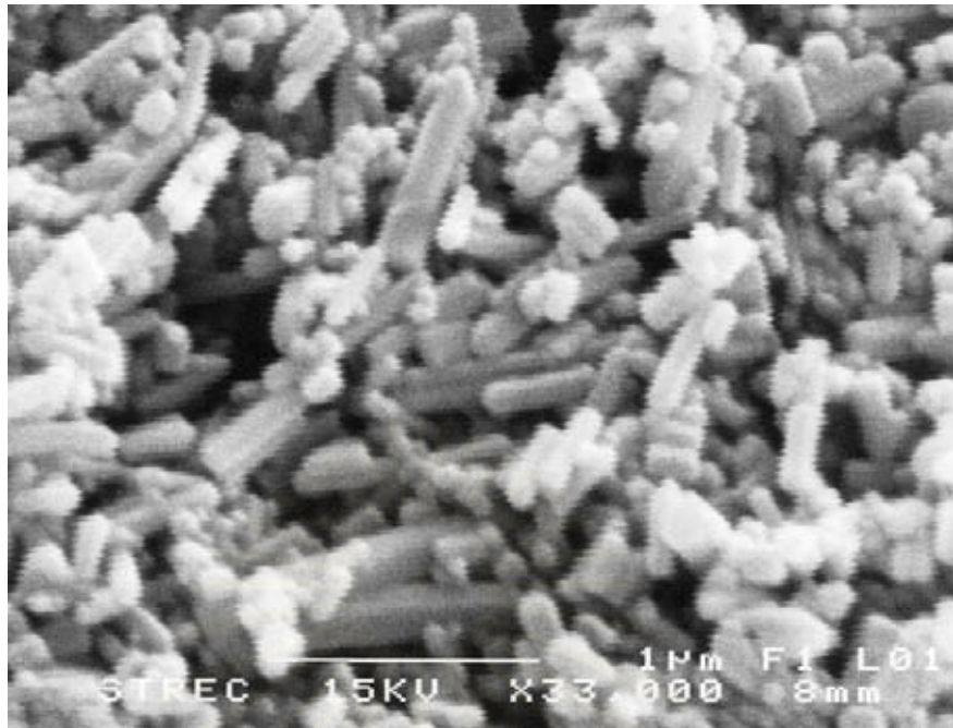
Figure 5.44 SEM image of ZnO nanoparticles as-synthesized in 1-octanol at 250 °C for 2 h by using zinc acetate 10 g.
