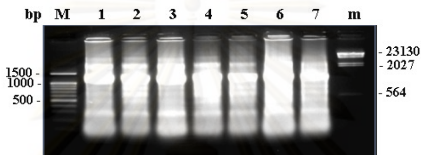
Figure 3.35 A 1.2% ethidium bromide-stained agarose gel showing the quality of total RNA extracted from testes of male P. monodon broodstock. Lanes M and m = a 100 bp DNA ladder and \lambda -Hind III, respectively. Lanes 1-7 = total RNA from different individuals of P. monodon .
