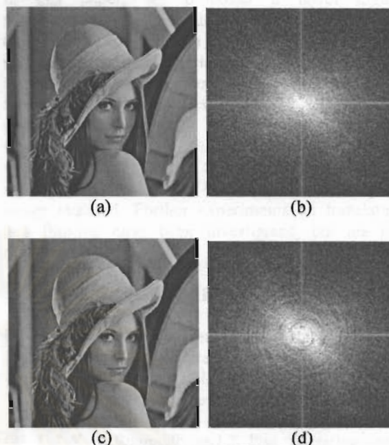
Fig. 2 (a) Original image and (b) its Fourier spectrum. (c) Watermarked image and (d) its Fourier spectrum.
