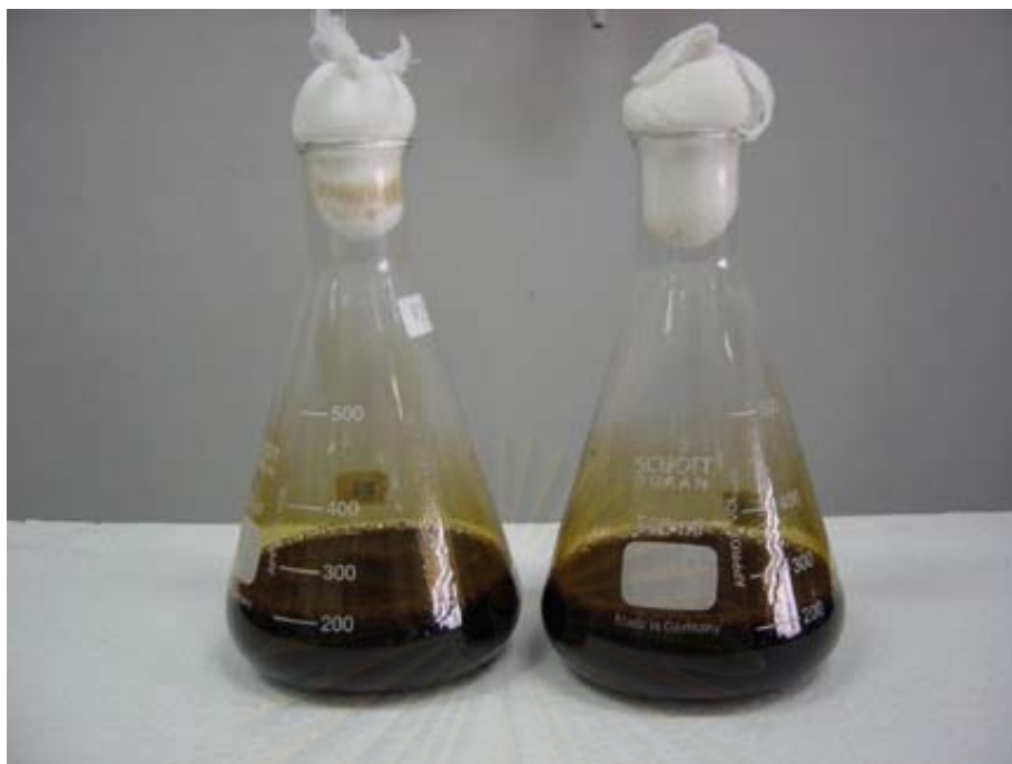
Figure 3.2 Saccharomyces cerevisiae M30 in 500 mL Erlenmeyer flasks containing 250 mL of the prepared fermentation media
