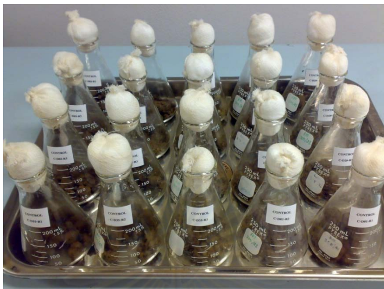
Figure 3.3 Microcosm set in sterilized flasks for the experiments.
