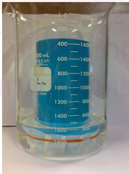
Figure B.1 Water holding capacity apparatus.
