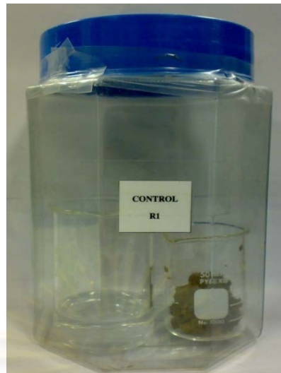
Figure 3.7 A closed chamber for CO 2 trapped contains a sample soil microcosm and a beaker of 0.05 N NaOH.
