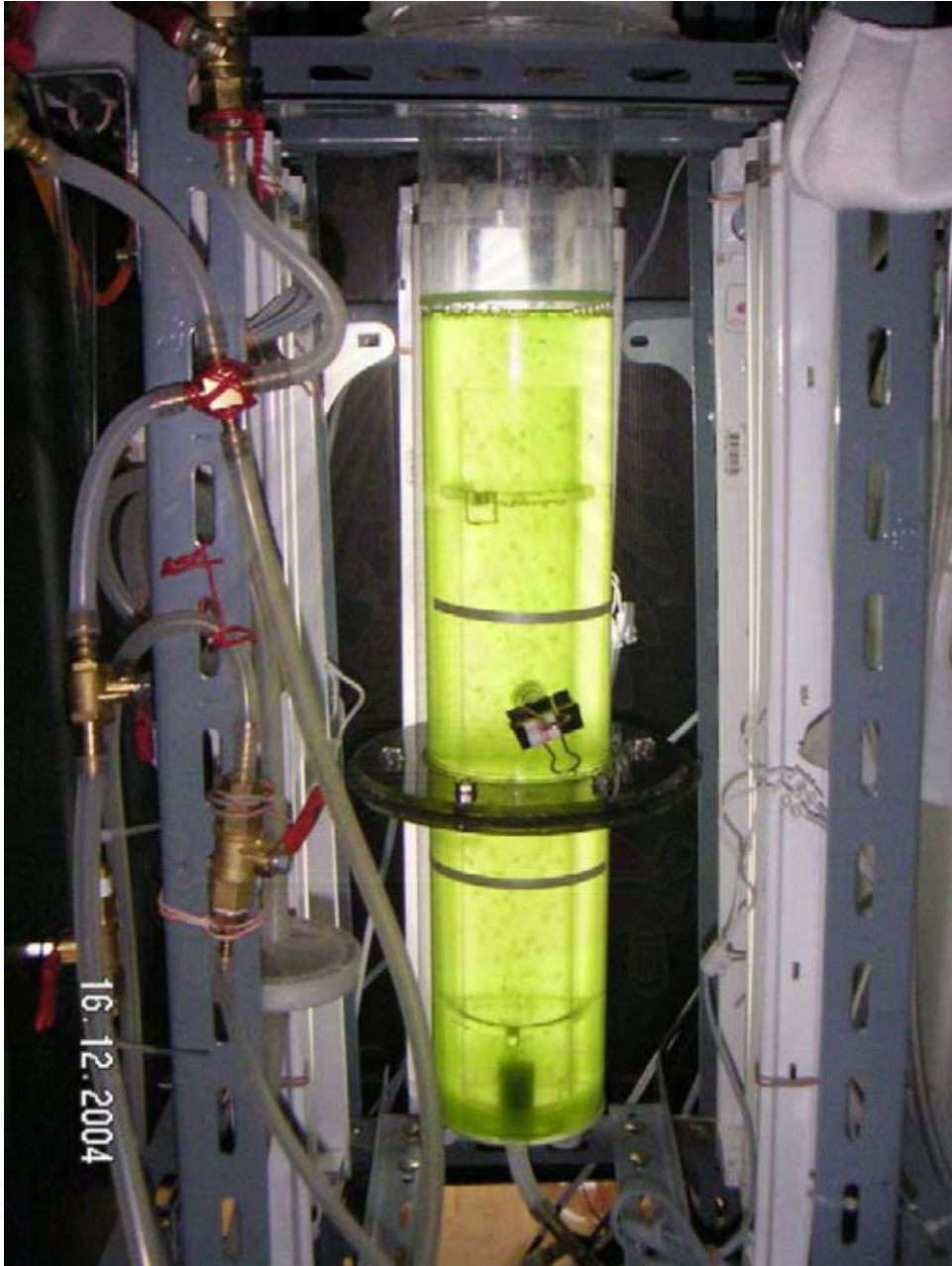
Figure 4.18(a) Cultivation of H. pluvialis in airlift bioreactor: growth stage
