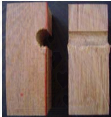
Figure 4.2 Wood crushing around the fastener hole
