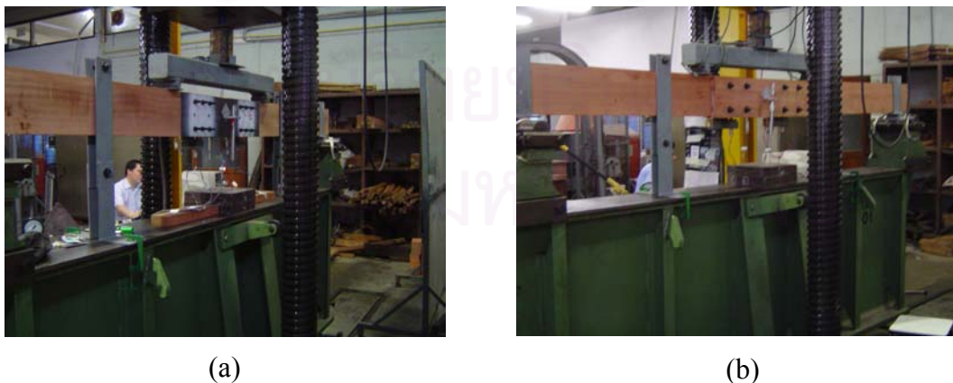
Figure 4.11 Multiple-bolt connections under investigation: (a) steel to wood connection, (b) wood to wood connection
