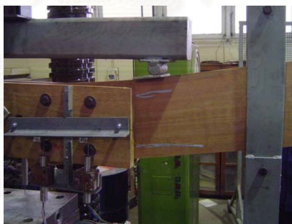
Figure 4.12 Joint rotation of experiment (specimen WW6V)
