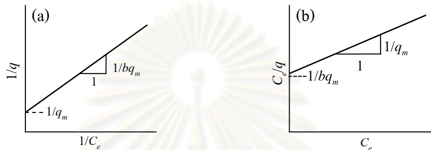
Figure 2.19 (a) Conventional linear form of Langmuir adsorption isotherm and (b) modified form of Langmuir adsorption isotherm emphasizing higher concentration data [90].
