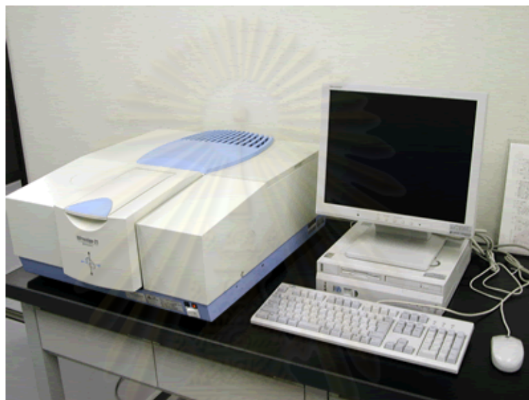
Figure 4.12 Fourier transform-infrared spectroscopy ( Shimadzu )
