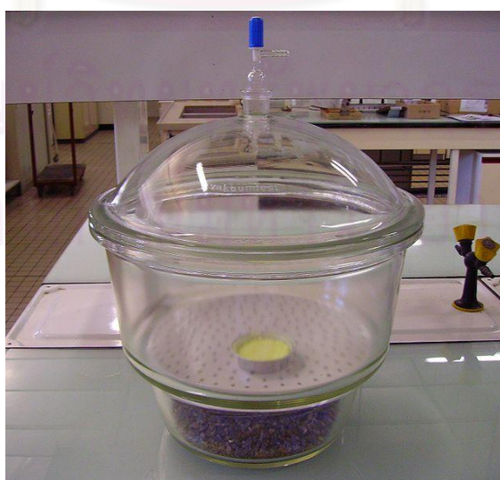
Figure 4.6 The desiccator for storage of CMS particles
