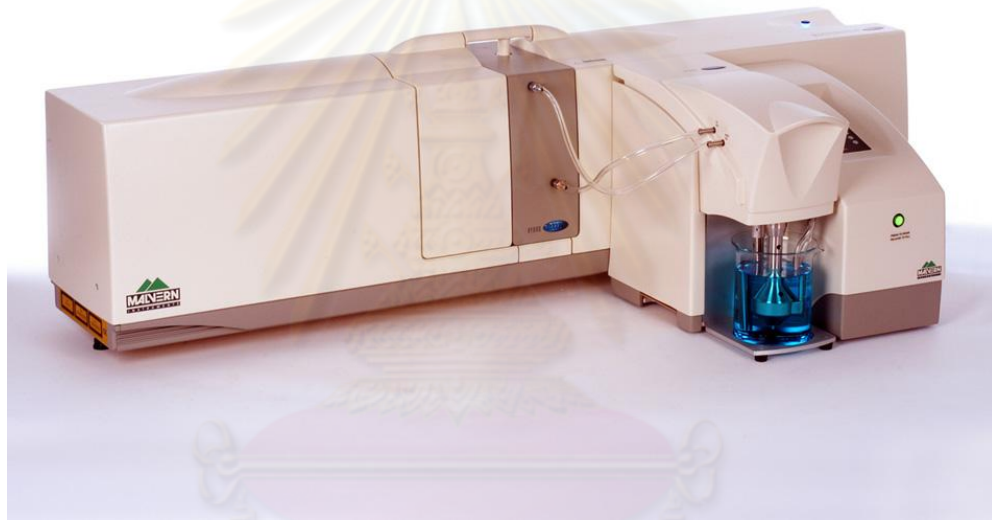
Figure 4.10 Laser scattering analyzer ( Mastersizer 2000: Malvern, United Kingdom )
