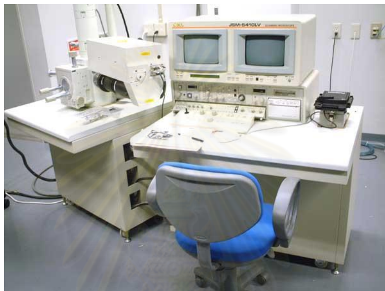
Figure 4.11 Scanning electron microscope (SEM, JEOL: JSM-5410LV, Japan)
