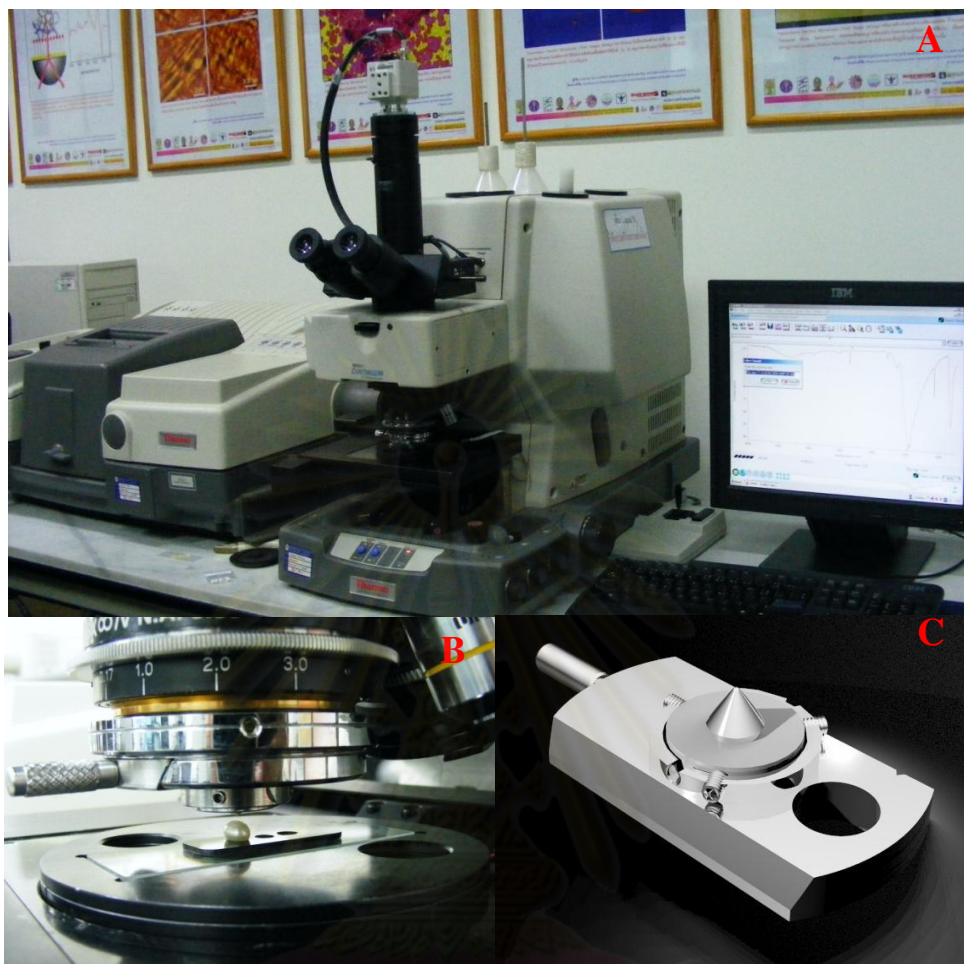
Figure 3.5 ATR FT-IR microspectroscopy: (A) Continuum™ infrared microscope attached to the Nicolet 6700 FT-IR spectrometer, (B) the holder of pearl and the slide-on Ge \mu IRE is fixed on the position of slide-on housing on the infrared objective, and (C) Homemade slide-on Ge \mu IRE.
