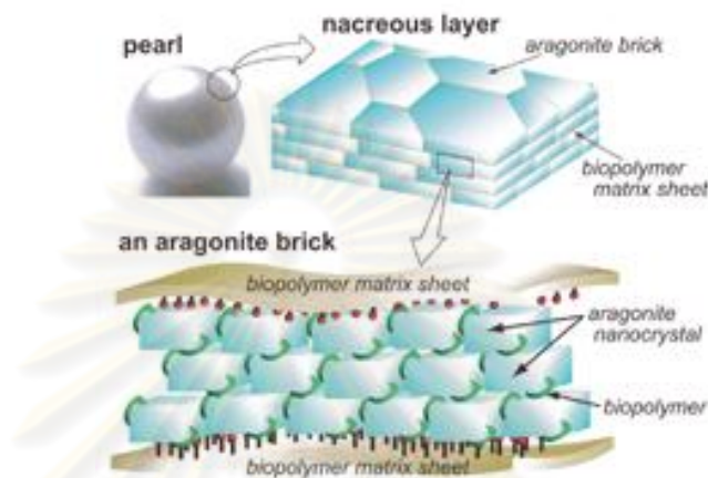
Figure 2.1 Structural assembly of pearl consisting of aragonite nanocrystal glued together by conchiolin protein (biopolymer) [20]
