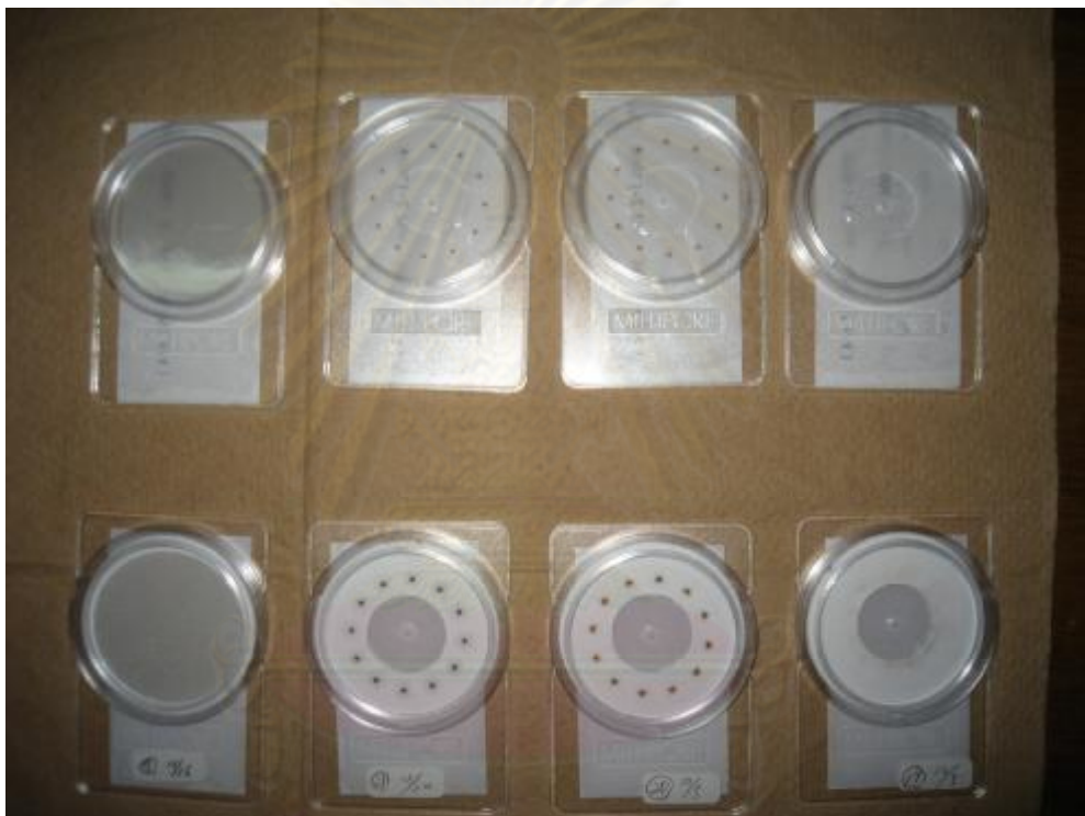
Figure 3.3 The filters were used in this study (top row: the polycarbonate filters (PC); bottom row: the quartz fiber filters (QF))
