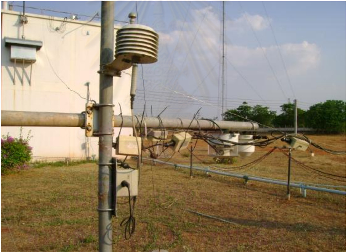
Figure 3.4 The instruments which measure the temperatures and air pressures at the Observatory
