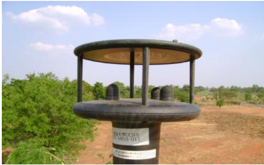
Figure 3.5 The instrument which measures wind speed and wind direction at the Observatory
