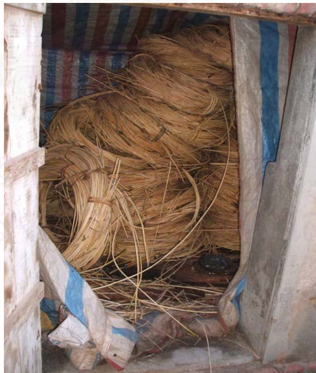
Figure 3 Rattan Bleaching smoked in sulfur dioxide room
