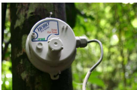
Figure 4.9 Air temperature data logger
