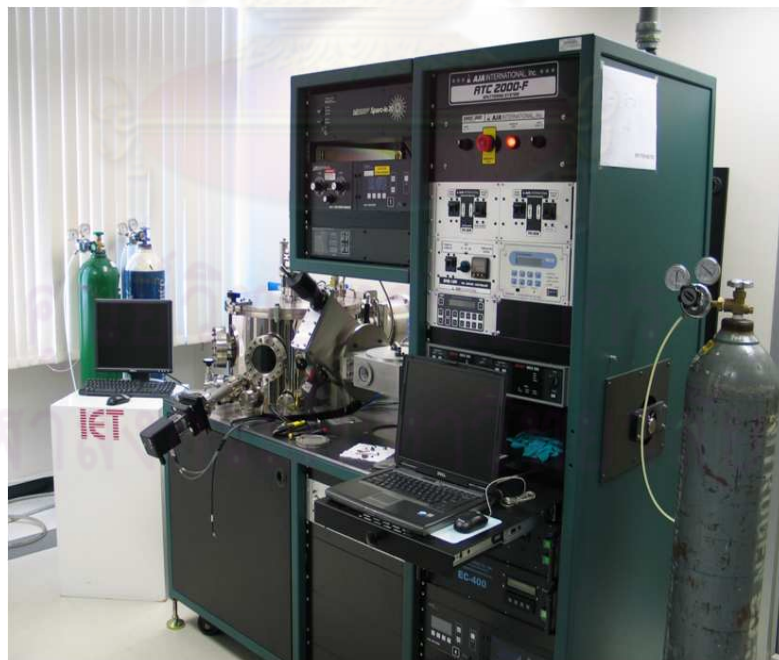
Figure 3.2: Schematic of AJA the sputtering system
