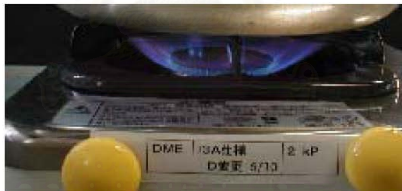
(c) 13A specification, damper opening : 5/10
