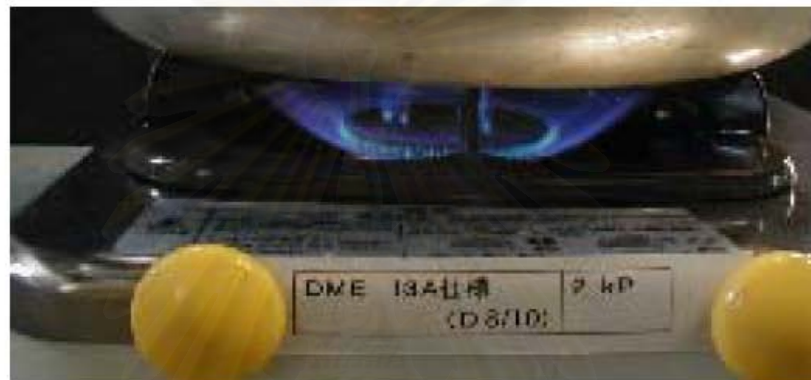
(b) 13A specification, damper opening : 8/10
