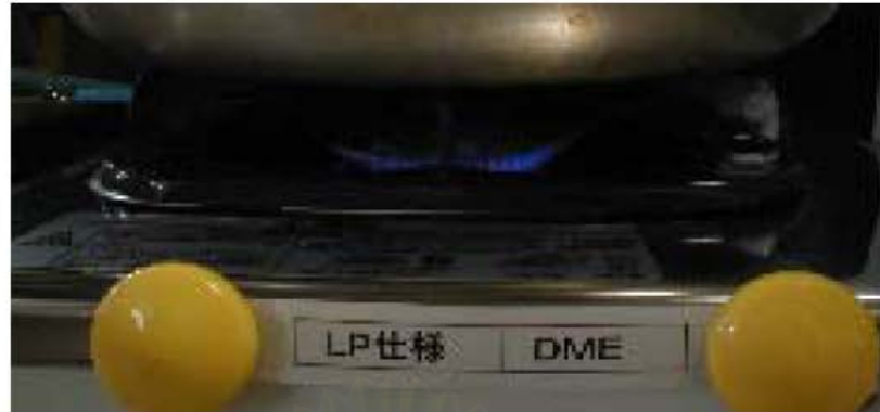
(a) LPG specification, damper opening : fixed
