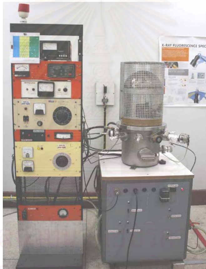
Figure 3.23: The used equipment to evaporate Ohmic contact.
