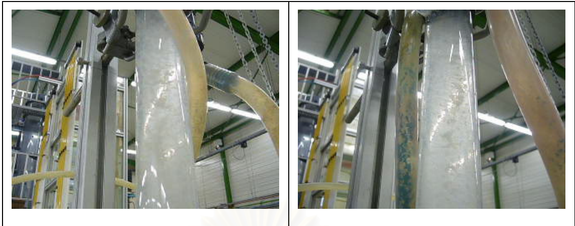
Figure IV-27. Separation lines in the hydrocyclone (HC3)
