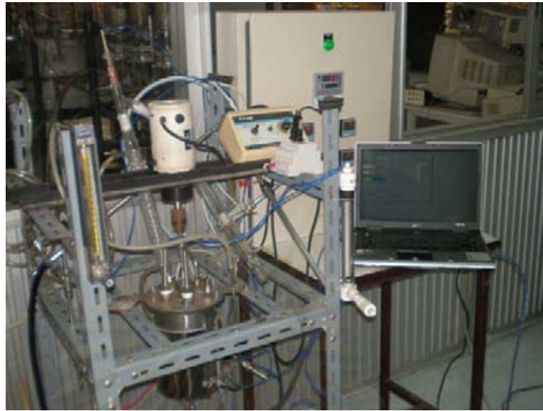
Figure 4.2 Batch polymerization reactor system which was used in this research
