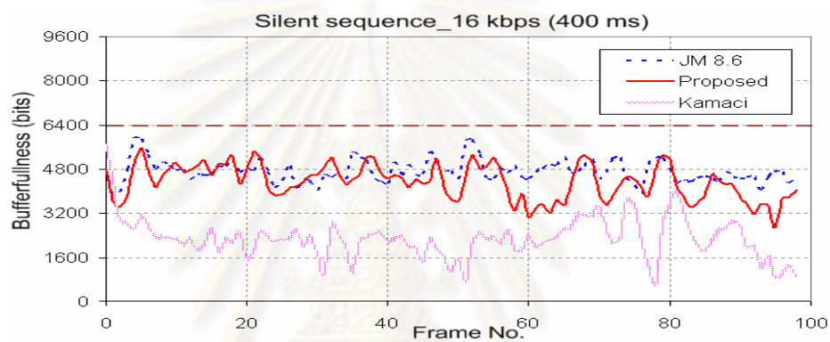
(a) Buffer fullness level (bits) at each frame with maximum delay constraint (dashed line) of Silent sequence.
