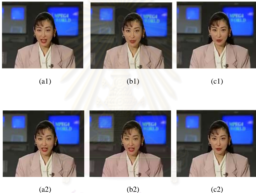
Figure 5.28 (a1)-(c1) show frames 40,41,42, respectively, of test sequence “Akiyo” coded with our proposed rate control scheme at 32 kbps , (a2)-(c2) are the same frames but coded with H.264 JM 8.6 rate control. Frame (b2) are identical with frame (a2) , because JM 8.6 rate control skipped one frame after coding frame (a2) since encoder buffer fullness was higher than maximum buffer size and (a2) was repeated at the encoder side to generated next frame.
