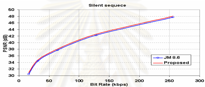
(f) Average PSNR versus bit rate in each frame for Silent sequence
