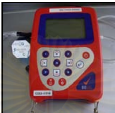
(a) Gas detector (Biogas check)
