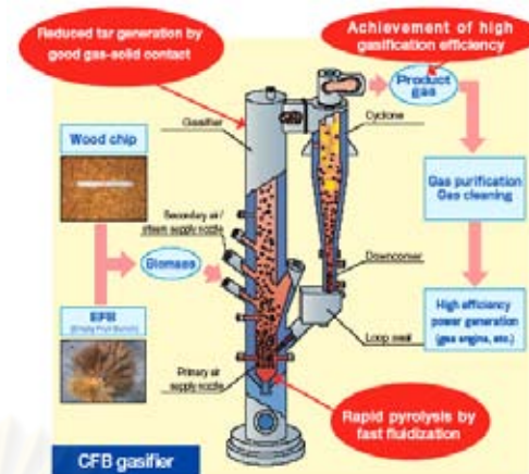
(ง) Fluidized bed gasifier
