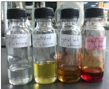
Figure 3.10 Hammett indicators used for measurement of acid strength.
