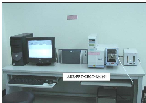
Figure 3.6 Perkin-Elmer Pyris Diamond thermogravimetric/Differential thermal analyzer.
