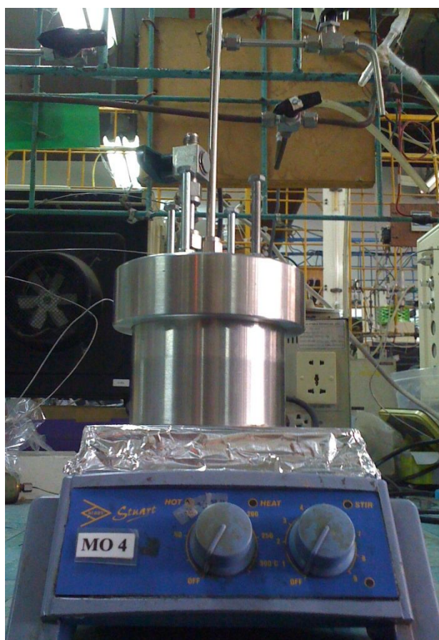
Figure 3.4 The experimental setup for autoclave reactor.
