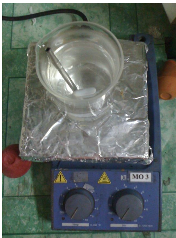
Figure 3.2 The experimental setup for the study of the solubility of benzene.
