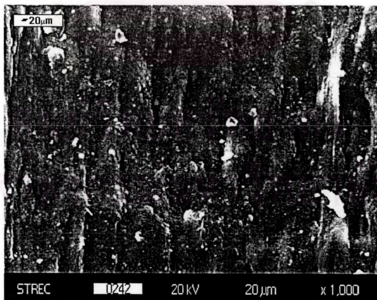
Figure 4.27 SEM micrograph of R-PVCOPS with CaCO 3 /talc 10 phr at 1,000X magnification
