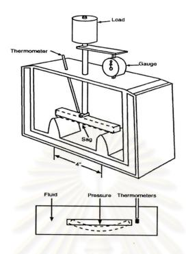
Figure 3.5 Schematic dimension of HDT test machine and specimen.
