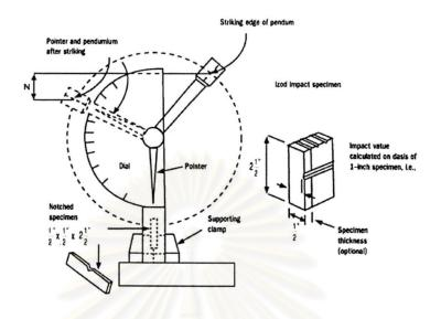
Figure 3.2 Schematic dimension of Izod Impact test machine and specimen
