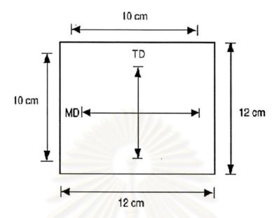
Figure 3.4 Schematic dimension of shrinkage test specimen
