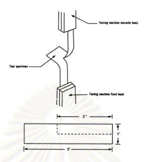
Figure 3.3 Schematic dimension of universal tester and specimen dimension
