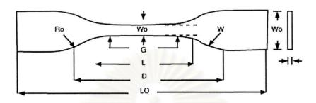
Figure 3.1 Schematic dimension of tensile test specimen
